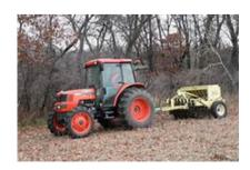
Working width 10 ft. Overall width 10 ft. 3 in. Weight 7000 lbs.
